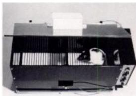
Stainless steel shuttle boxes. Easily sterilizable. System of 1 to 16 boxes controlled by IBM-PC. Shock/light/sound controlled by software. Infrared pass no pass sensors.
