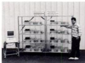
System of 1 to 8 mazes controlled by IBM-PC, supplied with software. Animal location is monitored by multiple IR beams.
