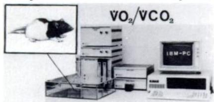
Open circuit "indirect calorimetry" method. Continuous measurement over 24 hrs. Totally computerized complete system for 1 to 4 animal cages, utilizes IBM-PC computer. High accuracy: 1%. Continuous airflow system. Also can measure relative tidal volume. Prints STP values in periodic intervals.
