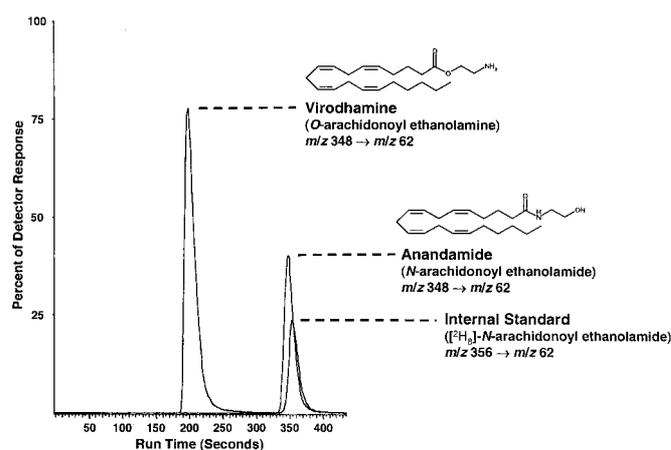
**Fig. 1.** LC APCI-MS-MS quantification of anandamide and virodhamine. Using *m/z* 348 ( $[\text{M} + \text{H}]^+$ ) as a precursor ion and *m/z* 62 as a product ion in a selected reaction monitoring mode, both anandamide and virodhamine concentrations were quantified. Anandamide and virodhamine were easily separated chromatographically using a C-18 column under isocratic conditions.
